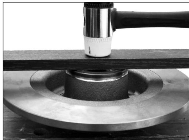
**\*\* Failure to apply the correct pre-load to the bearing may result in excessive play, noise, overheating and premature bearing failure.**
